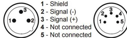
If you are using the standard DMX controllers, you can connect the DMX output of the controller directly with the DMX input of the first fixture in the DMX-chain. If you wish to connect DMX-controllers with other XLR-outputs, you need to use adapter-cables.
